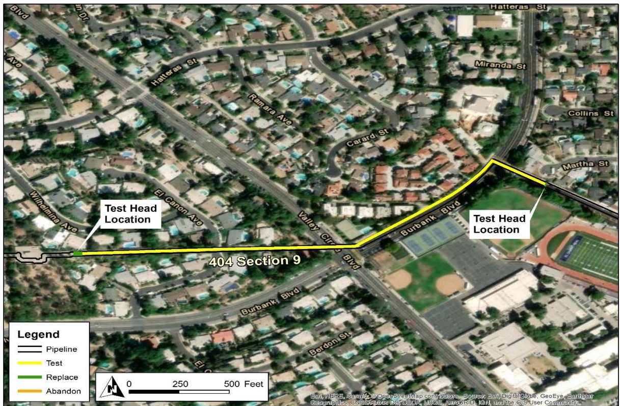
Figure 12: Satellite Image of Line 404 Section 9 Hydrotest Project
