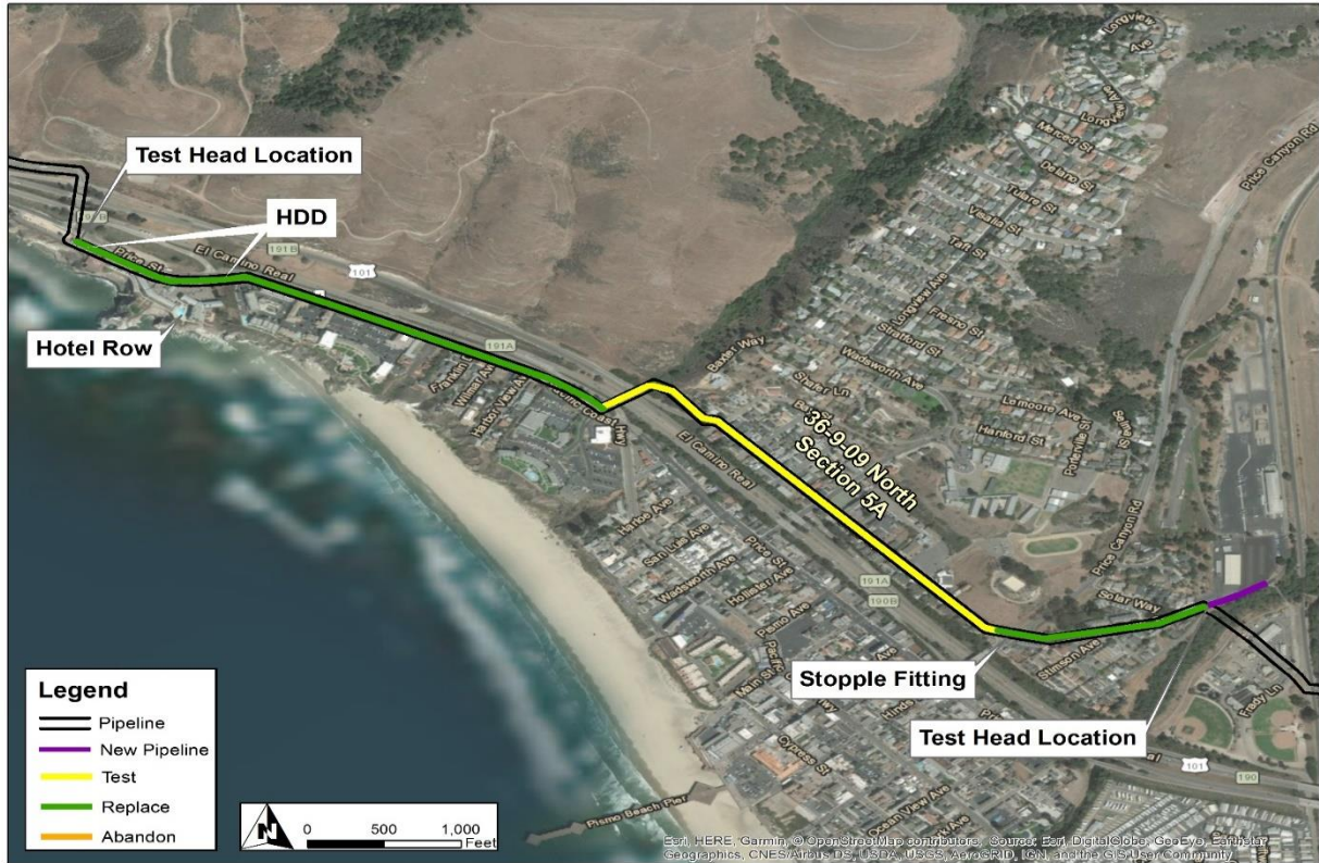
Figure 2: Satellite Image of Supply Line 36-9-09 North Section 5A Hydrotest and Replacement Project
